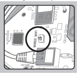
Remove the device lid by removing the two screws on the cover. To clear any previous Wi-Fi settings, toggle the Wired-Wi-Fi switch. Set the switch to the desired mode. Proceed to step 3.1 or 3.2 to reprogram the Wi-Fi settings
