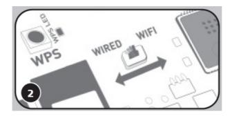
The iQ30 will start Wi-Fi setup mode when the WIRED / WI-FI switch is set to Wi-Fi and its memory has been cleared. To clear the memory, toggle the switch and leave it in the Wi-Fi position.
