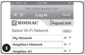
Signal strength depends on your router and the mounting location of the iQ30 web-connect device. Use the Hotspot method to evaluate (See Section 3.1). If you move the router closer and signal still not strong, consider installing a Wi-Fi range extender, Wi-Fi repeater, or another type of router. You may also install an app on your smart phone (e.g., Wi-Fi Analyzer or Wi-Fi Sweetspots) to check your signal strength and bandwidth.
