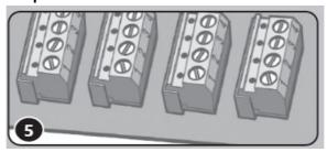
A maximum of two (2) RS485 cables can be connected per RS485 connector. To connect additional RS485 devices, a Multiplex Board may be required.
