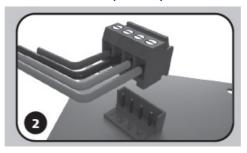
NOTE: Do not connect more than two RS485 cables per red terminal bar3
