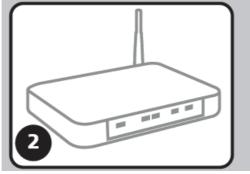
3. Press and release the WPS button on the web-connect device. The small yellow LED next to the button will start blinking slowly.
