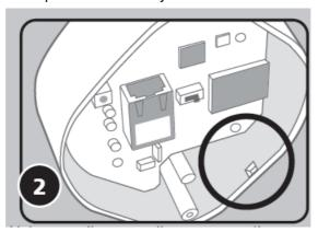
3. Insert the ethernet cable into the ethernet port and wrap the cable inside the device and out of the break-away. To reduce electromagnetic noise, wrap ethernet cable twice around a snap-on ferrite bead exterior to the device, as shown in figure (3). Contact Zodiac Pool Systems LLC Customer Service for a Ferrite Kit (PN# R0914600), provided free of charge. (Ferrite Specs: Fair-Rite PN# 0443806406)
