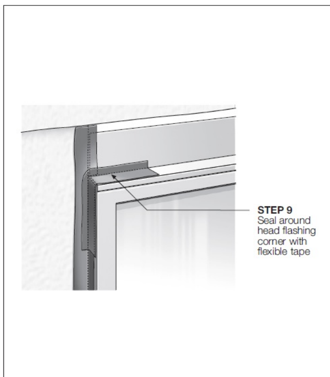
FIGURE 46 INSTALLATION OF WINDOW
