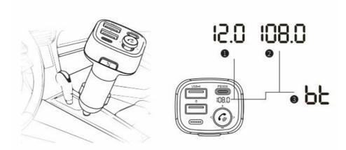
3. Long press the multifunction button, then adjust the transmitter to the same frequency on the car by pushing the Multifunction button left or right when the LED displays FM frequency.
