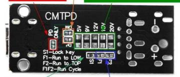
S1 is the key lock setting 1 after the short connection, the switching voltage should be unlocked, and the unlocking method is to press and power on the key F1 shorting: Power on automatically polls to the highest voltage and then holds to 5V, and the LED will show the corresponding supported voltage. F2 shorted: shorted to F1 but maintained at the highest supported voltage. F1F2 simultaneously shorted: for infinite loop
