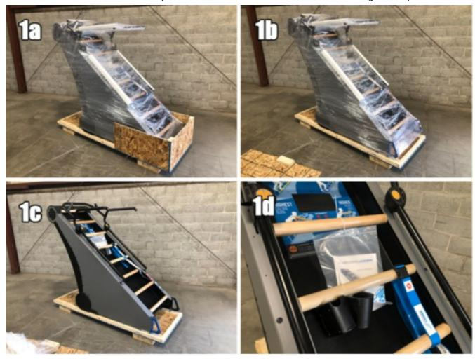
2. Unbolt the ladder from the pallet, secure the stabilizer bars so they are stowed inside the unit and roll the unit
