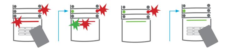
A triggered alarm in progress is indicated by a rapidly flashing red segment button and a backlit indication button. You need to authorize yourself using the keypad in order to terminate the alarm. The section remains set, a rapidly flashing red segment button indicates the alarm memory. Indication will keep on flashing even after the system has been unset.
