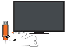
3. Remove the other liner. Firmly press the USB™ connector to the desired location for 30 seconds.
