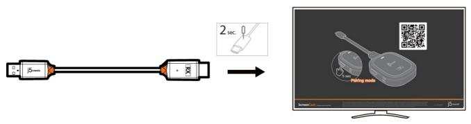
Press the reset button of receiver again for 5 seconds to enter pairing mode.
