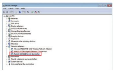
**Note:** If you want to confirm if the installation is correct, go to Device Manager and click the network adapter option to confirm. If the device name of "Realtek USBTM GbE Family Controller" is displayed, the external network adapter is installed correctly.
