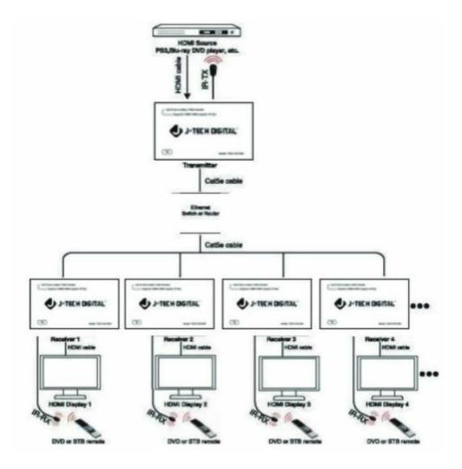
Note: Connect HDMI Transmitter port and Receiver ports to the Ethernet Switch
