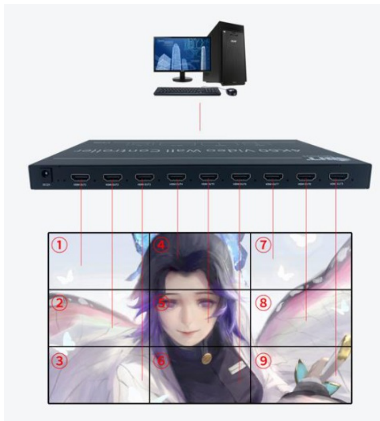
3×3 mode front panel wiring diagram (5760×3240@60Hz)
