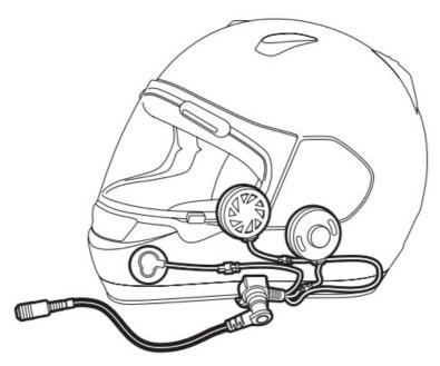
1. Most full-face style helmets have cheek pads or a complete nose section that can be removed. Carefully do so at this time, paying special attention so as not to break or damage any of the polystyrene parts and also remove the soft fabric lining material around the cheek pads.
