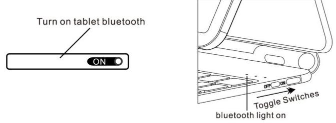
3. The bluetooth light of the keyboard flashes, click "Bluetooth Keyboard" in the "Other Devices" of the tablet to enter the window and click "Pair", after the pairing is successful, the blue light goes out.
