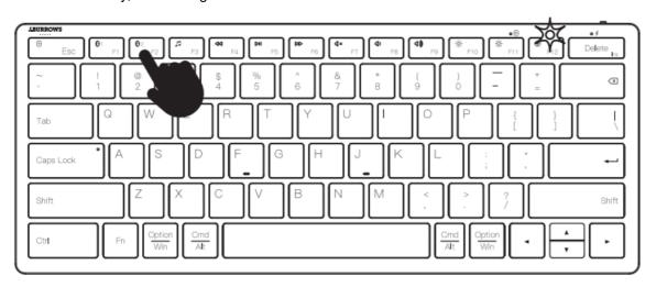
• Hold the BT2 key for more than 3 seconds until the blue light flashes quickly.
