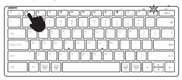
• Hold the BT1 key for more than 3 seconds until the red light flashes quickly.
