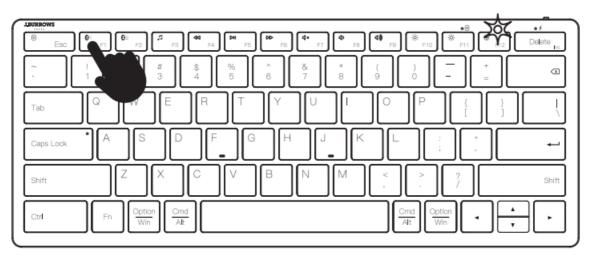
Now it is in Bluetooth pairing mode. Go to Bluetooth setting on your device and select Elite **MK350-KB** for keyboard, Elite **MK350-MS** for mouse. Follow the onscreen instructions to complete the pairing. The light will turn off once Bluetooth pairing is successful
