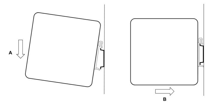
The SecureEdge Pro is mounted on a standard DIN rail. Hang the device on the rail and (A) push the unit down and (B) towards the DIN rail until you feel a click.
