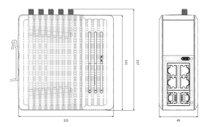
The SecureEdge Pro is designed to be cooled using natural convection. For proper cooling, you must provide a clearance of at least 35 mm above and below the device. Also, allow at least 35 mm of depth between the front of the device and the inside of the control cabinet.
