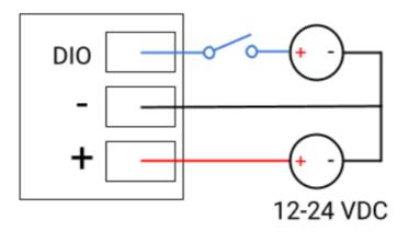
The Digital Input provides a way to locally manage SecureEdge Pro's VPN connection (ON/OFF). The wiring for proper operation of Digital Input (DI) is depicted in the image above.
