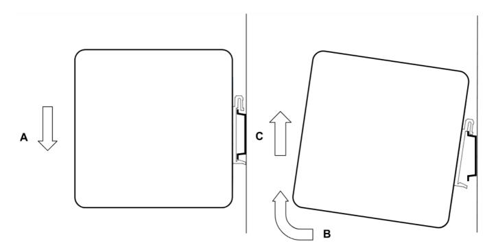
To remove the unit, (A) push the device down, (B) pull and rotate the device up and (C) lift off the rail.
