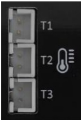
Figure 3: NTC sensors inputs T1-T3
