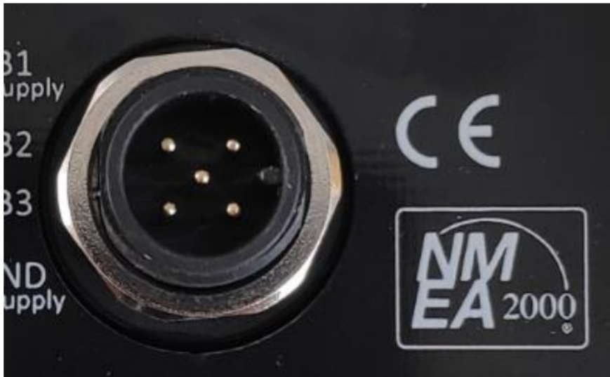
• Figure 5: NMEA2000 M12 Male connector pinout (view from unit side)
