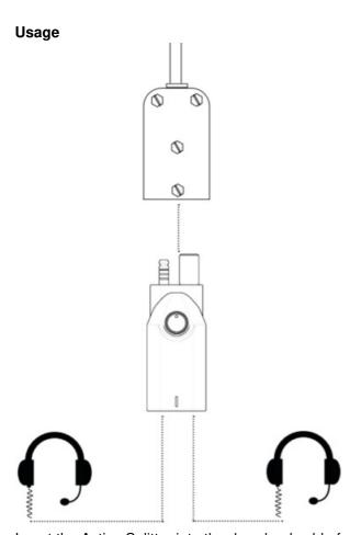
Insert the Active Splitter into the downlead cable from your CAP (Communication Access Panel).
