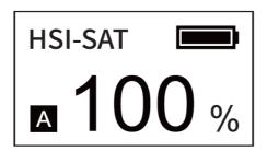
Tap the button to switch Brightness(INT), HUE, or SAT, and tap or press and hold to the value. Brightness range:
