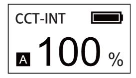
Tap the button to switch between brightness(INT) or color temperature(CT), and tap or press and hold
