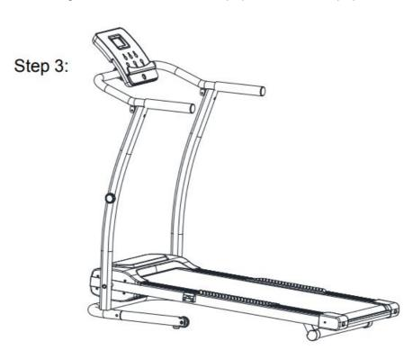
Pull the (48)Fixed knob when putting down the treadmill. When pulling the (48)Fixed knob, you must hold the running platform well and make sure that the running platform is flat on the ground to release your hand.
