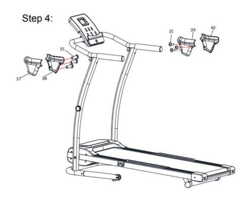
Will (37) (38), (39) (40) cover fixed in (3) tables and columns (1) joint, with wrench to tighten the screw (21) (74).
