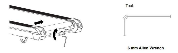
If the running belt is shifting to the right, then turn the right adjustment bolt 1/4 turn clockwise, and the belt should start to correct itself. Keep turning the adjustment bolts until the running belt is properly cantered.
