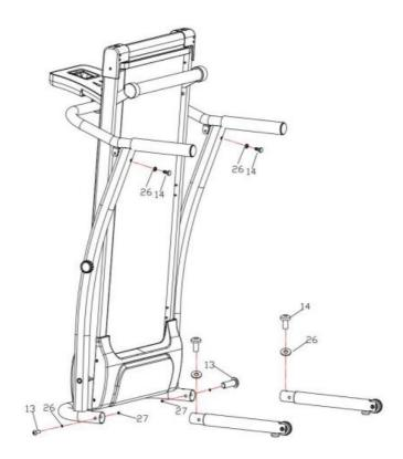
Put the treadmill on the ground, use pull pin fixing the running deck, then use the Allen Wrench(32) to lock Hexagon Socket Button Head Bolt(13), Washer26), Nylon Nut(27) with the Base lengthening tube(5), And then lock the handrail with the Hexagon Socket Button Head Bolt(14) and the Washer(26).
