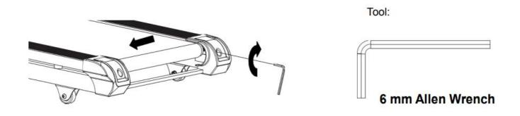
If the running belt is slipping during use, turn off and unplug the treadmill. Using the 6 mm Allen Wrench provided, turn both left and right rear roller adjustment bolts 1/4 turn clockwise, then turn the main power switch back on and run the treadmill at a speed of 8-10 KPH. Run on to the running belt to determine if the belt is still slipping. Repeat this procedure until the belt no longer slips.
