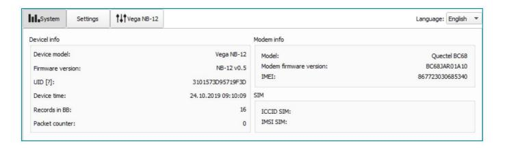
**Device info** – the configurator reads information about the device model, its firmware and automatically corrects the device's time when connected to it. In that block you can find out the number of records in the black box and the number of packets sent by the device.
