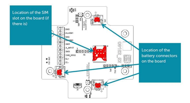
Vega NB-12 modem powered by the one, two or three batteries which comes with1. There are equivalent connectors located on the board. After battery connection to one of connectors, the device loaded and switched to the 'Sleep' mode until the communication session according with the schedule.
