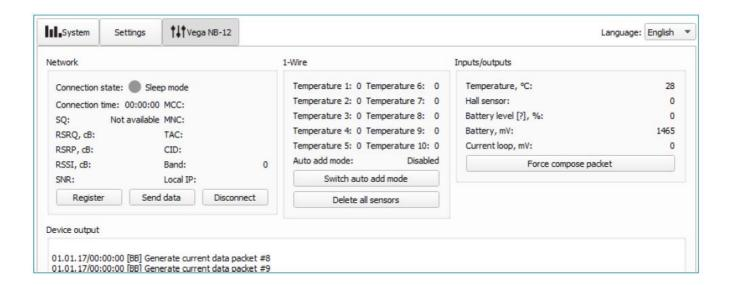
**Network** – displays the current parameters of the connection and allows to control it. Buttons in this block have logic like INIT button on the board.
