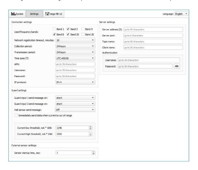
Connection settings – a group of parameters set up the data collection and transmitting.
