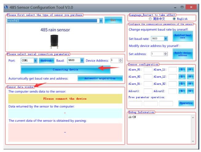
6. Then if the sensor is well connected, the user can see the data status on the "Sensor data window"
