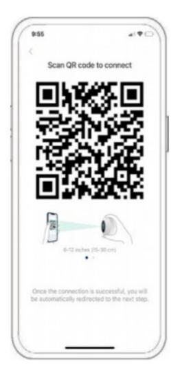
2. After pressing the camera switch for 3 seconds, the camera will turn on. At this moment, target the camera at the QR code of the mobile App, with a distance of about 20cm (about 7 inches) until the camera emits a "Di" sound, which represents the scanning is succeeded and the pairing is started.
