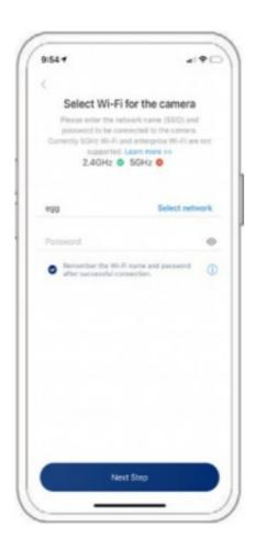
To ensure a longer distance connection, the camera only supports the 2.4Ghz Wi-Fi with stronger wall penetration capability and does not support Wi-Fi for enterprise- level authentication currently. Please ensure that the entered Wi-Fi meets the requirements. After completion, click "Continue" to generate the QR code for pairing the camera.
