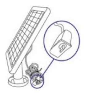
Insert the micro-USB plug into the micro-USB port on the camera. Ensure area is sealed with white weather proof
