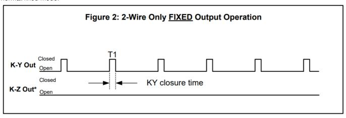
\*If the output is configured for Form A pulses the K-Z output is is not used. In Figure 2 above, the K-Z output is disabled, thus showing no pulses.
