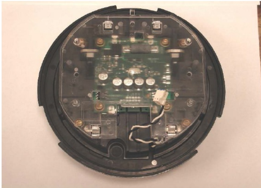
Meter Base with CAT3 module installed
