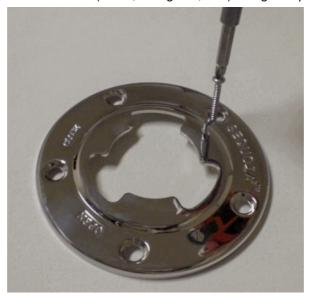
2. Mount the table base onto table top (customer provid-ed) using #10 phillips oval head screws. Make sure the weight of the table top is evenly supported over the table leg.
