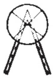
Do not bend right at solder joint
