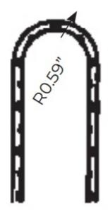
Do not twist more than 90° over the length of one 24V segment / Two 12V segments (4" total length)
