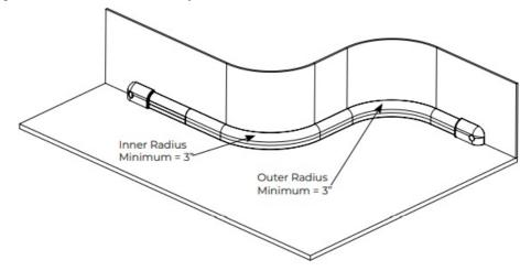
wire routing and access as well as any corner applications. The light can only be bent to a 3" radius, wrapping it around a corner at a tighter radius may damage the light and will void the warranty.
