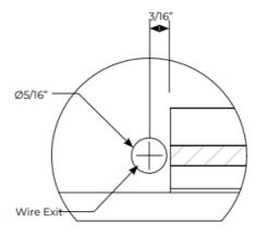
3. Clean the mounting surface using alcohol wipes (not provided). For more information on surface prep please review the 3M websites\*. Starting at the wire exit, begin removing the tape backing two to three feet at a time. Removing more backing may contaminate the adhesive. Carefully position the light and gently press it in place. Once the light is positioned properly push firmly in place to activate the pressure-sensitive adhesive. Allow 72 hours for full bond strength.
