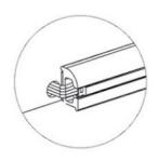
4. Place end caps on each end and use them as a template to mark the screw hole. Drill appropriate size holes for your application, making sure wires are clear of the hole before drilling. Install the screws to secure each end cap.
