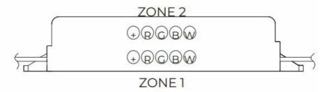
3. **TWO-ZONE WIRING DIAGRAMS:** Follow the wiring diagram below to wire the module to your system. Note: Maximum replacement fuse size is 20 amps.
