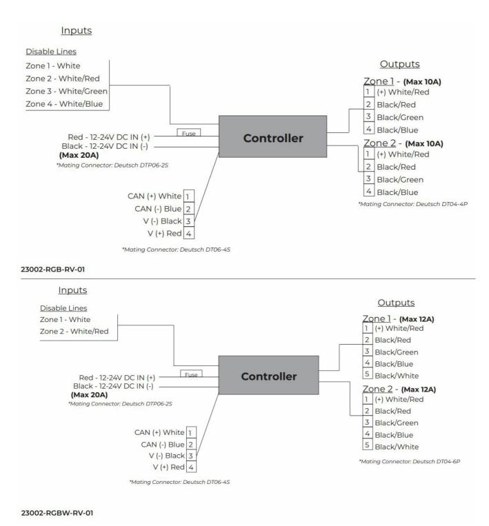
4. **FOUR-ZONE WIRING DIAGRAMS:** Follow the wiring diagram below to wire the module to your system. Note: Maximum replacement fuse size is 20 amps.
