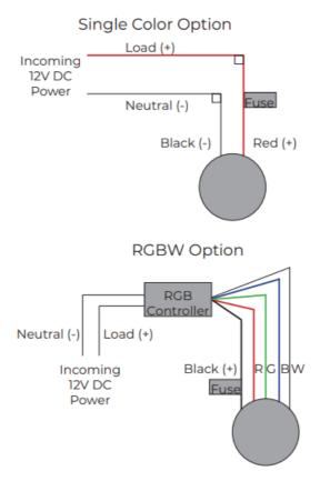
2. Wire the light based on the wiring diagram. Feed wires back into the hole and push the light in place. Use silicone sealant to hold it in place.
