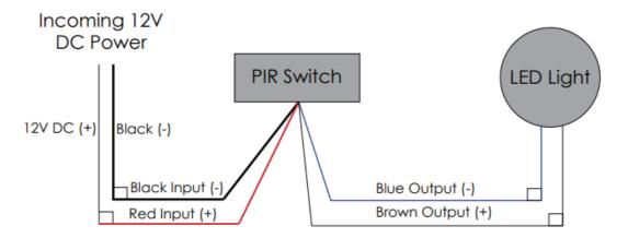
5. OPERATION: The PIR switch will turn on the lights when it senses motion and will turn off after three minutes if no motion is detected. The switch has a range of 120° and a distance of 3' from the center of the sensor.
