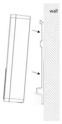
4. Fix the reader to the bracket with bracket screw IRD2M slim type reader
