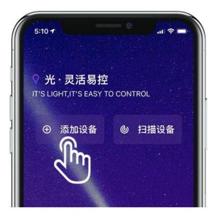
Confirm that the current mobile phone is connected to WiFi, and the App will automatically fill in the WiFi connection to the current mobile phone, you need to manually enter the password, click the connect button (note: 5GHz WiFi is not supported)
