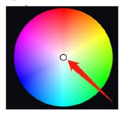
The color temperature adjustment belt can adjust the color temperature. The yellow side is a warm color, and the blue side is a cold color. After selecting the white light channel, the adjustment effect will be the best under the white light.
