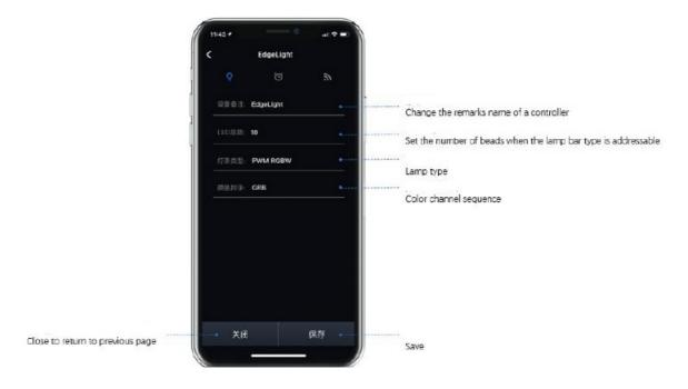
Timing setting: set the opening and closing time of the light bar
