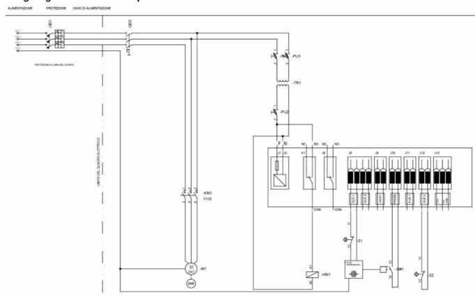
Wiring diagram UNI 2 C 230V 1ph
