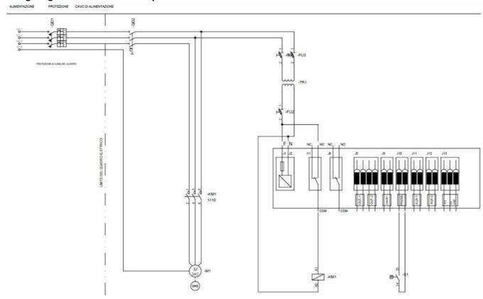
Wiring diagram UNI 2 E 230V 1ph
