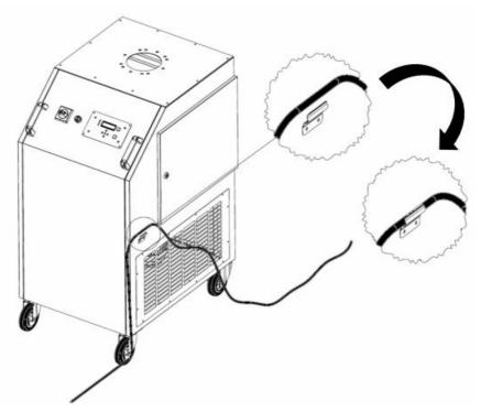
To ensure proper operation of the automatic Start / Stop device, it is essential that the ground cable of the welding unit is placed on the metal cabinet of the filter unit and locked in position by the special clamp. Check that the ground cable is well in contact with the metal cabinet of the unit, as shown in the figure.
