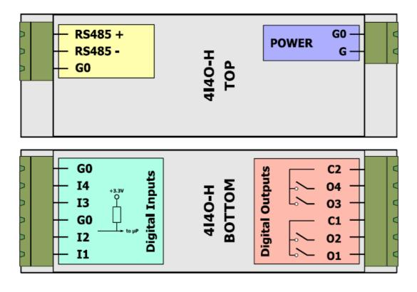
All G0 terminals are connected together internally
