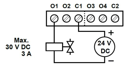
• Every CX terminal can be supplied by a different PELV/SELV source
