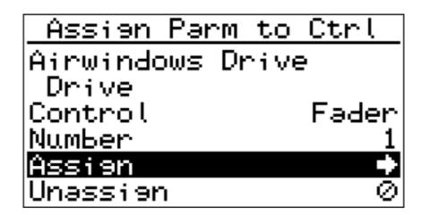
This screen appears after F4 is pressed on the Plugin Parameter Editor screen. The top two lines of the screen show the plugin name and the parameter name. The other fields are listed below.
