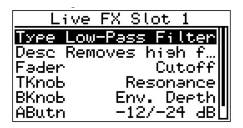
The top row selects the algorithm. The screen also includes a scrolling description of the algorithm and the parameters controlled by the fader, knobs, and buttons.
