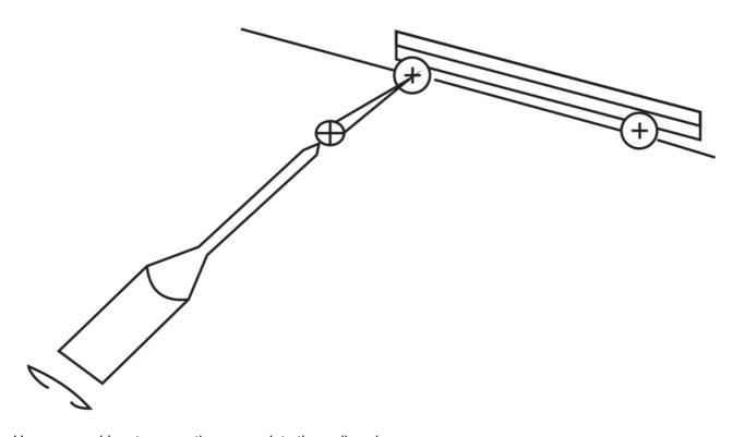
Use a screwdriver to screw the screws into the wall anchors.
