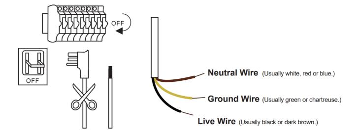
Cut the plug, connect the same color wire and tighten them (Disconnect power before hardwire).
