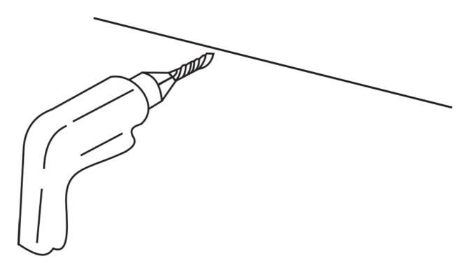
Use a electric drill to punch four holes at the marked spots.
