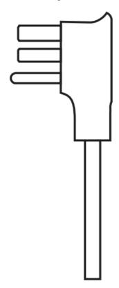
Insert the plug into the socket, keep the voltages between 110V and 120V. If the voltage exceeds 120V, please use transformer.
