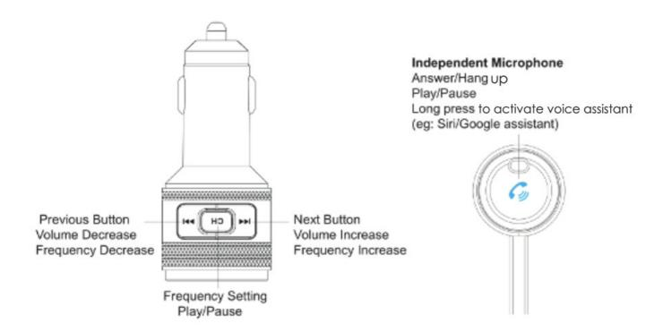
Press CH and hold till the frequency keep flashing, then press to increase the frequency and press to decrease the frequency.
