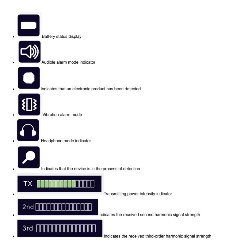
When a suspicious electronic device is detected in the target area, the second harmonic signal strength is significantly stronger than the third harmonic signal strength, and the electronic product icon is displayed on the screen.
