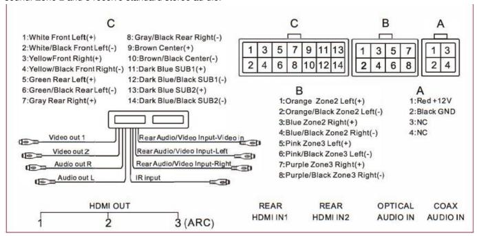
This unit has 1 Video Input, 2 Video outputs, 3 Audio inputs, 1 Digital/Optical input to allow users to enjoy entertainment from other sources such as Satellite Radio, VCR's, Digital Cameras, and Video Games for iPods and MP3 Players.
