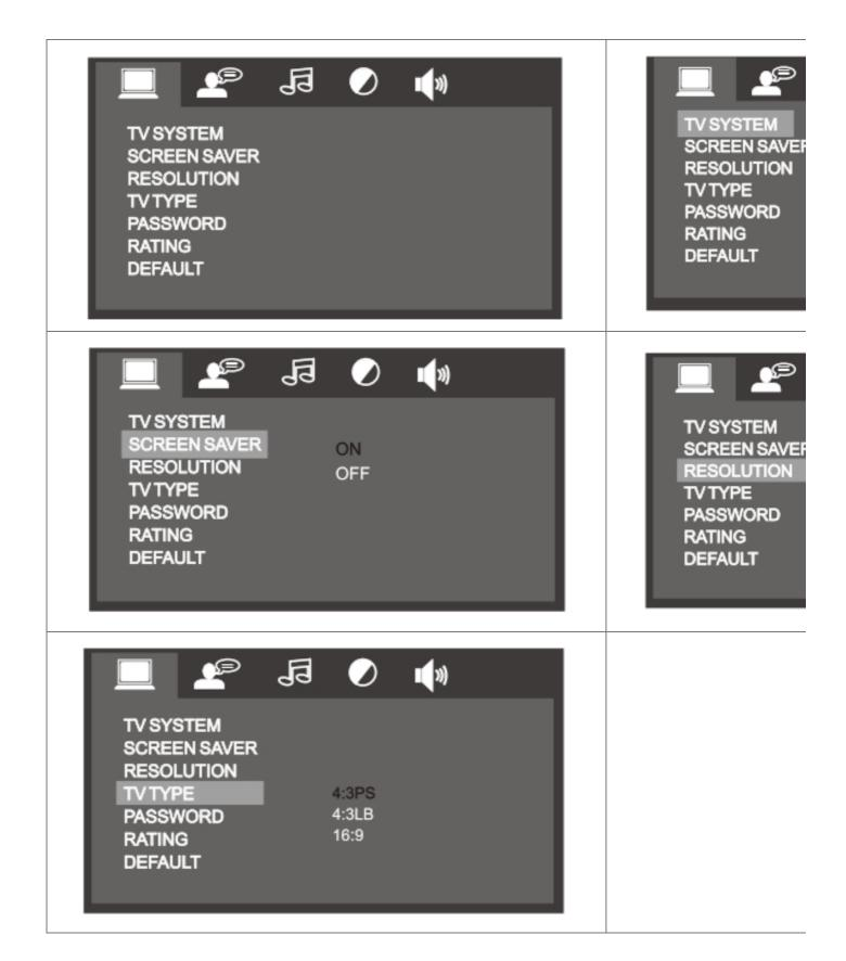
Press the "SETUP" button to activate the System Setup on-screen display Video Monitor Only menu. Use the NAVIGATION buttons to navigate the following OSD menu options.
