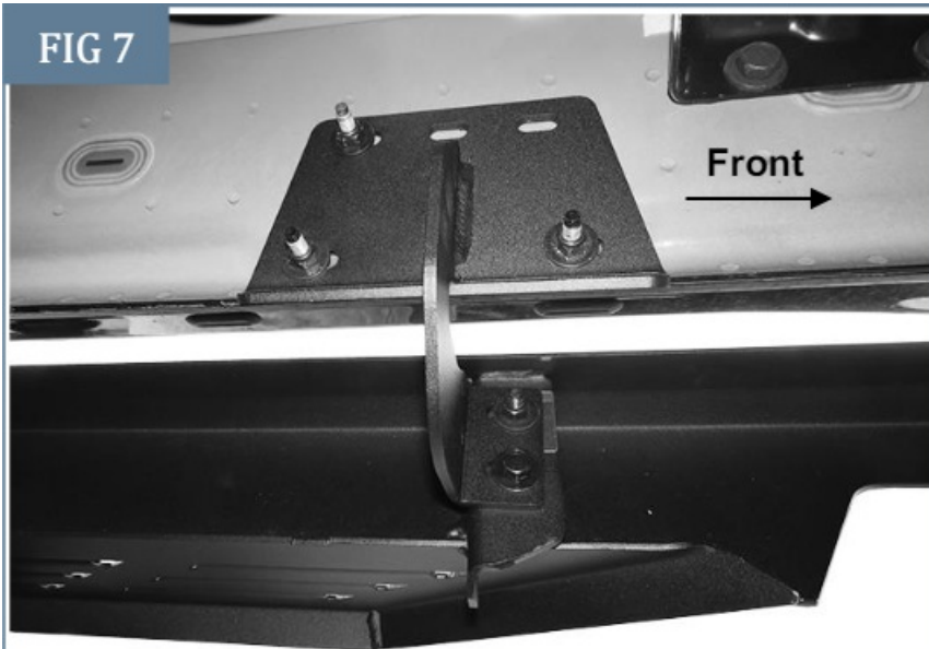
(Fig 7) Driver/Left Running Board attached to the front Mounting Bracket
