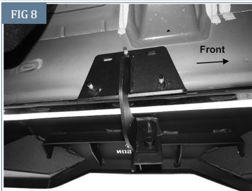
(Fig 8) Driver/Left Running Board attached to the center Mounting Bracket
