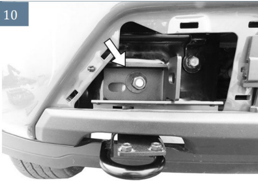
(Fig 10) Attach passenger/right Frame Bracket to Bolt Plate (arrow)
