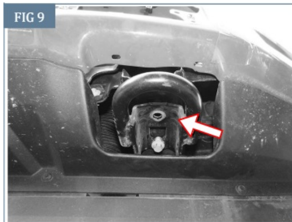
(Fig 9) Models with tow hooks, remove forward bolt and loosen but do not remove rear bolt to hold factory double nut plate in place in frame
