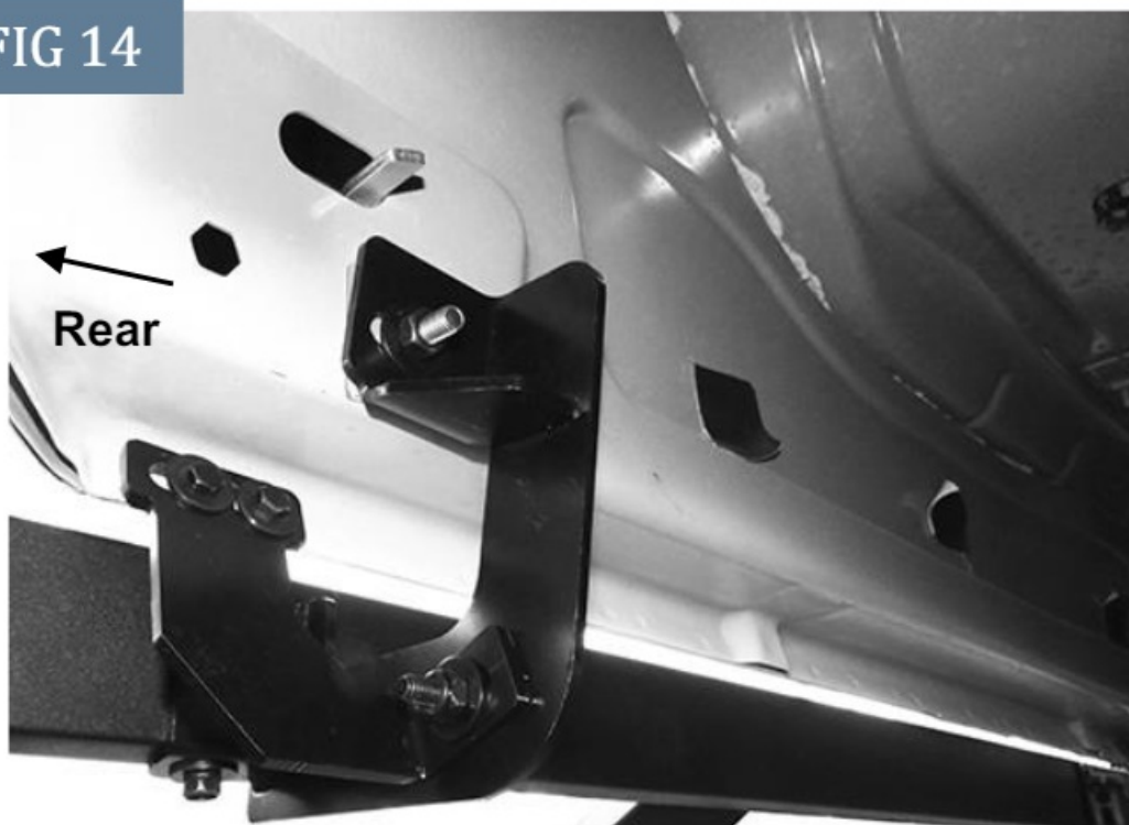
(Fig 14) Driver/left Side Step attached to Rear Brackets
