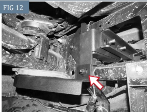
(Fig 12) Attach bent end of Support Bracket to back of Frame Bracket (arrow)
