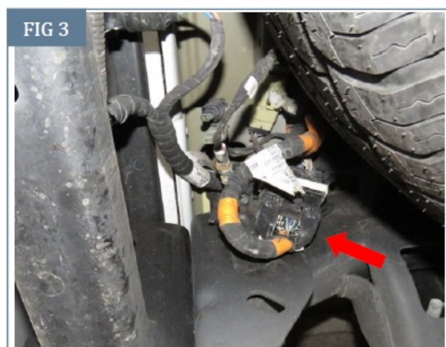
(Fig 3) Locate and remove wiring harnesses leading to bumper
