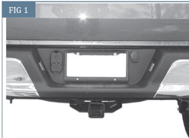
(Fig 1) Unplug and remove 7-wire trailer plug
