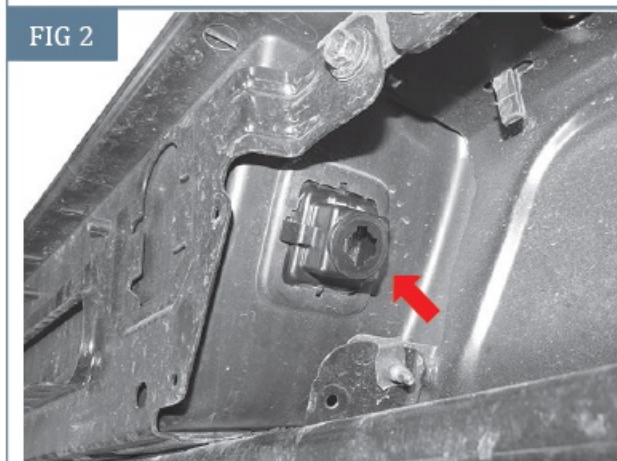
(Fig 2) Unplug license plate lights
