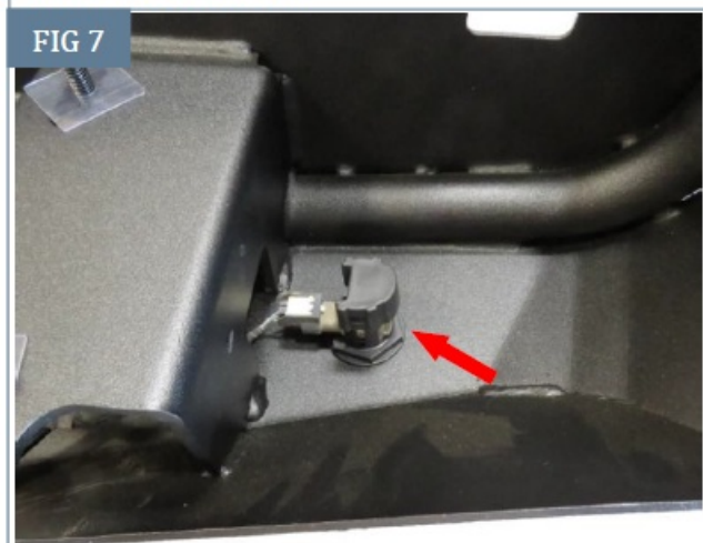
(Fig 7) Parking sensor installed
