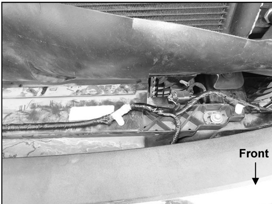
(Fig 15) F-150 Models. Locate the wiring harness to the sensor. From the plug, unwrap approximately 24" of the harness.
