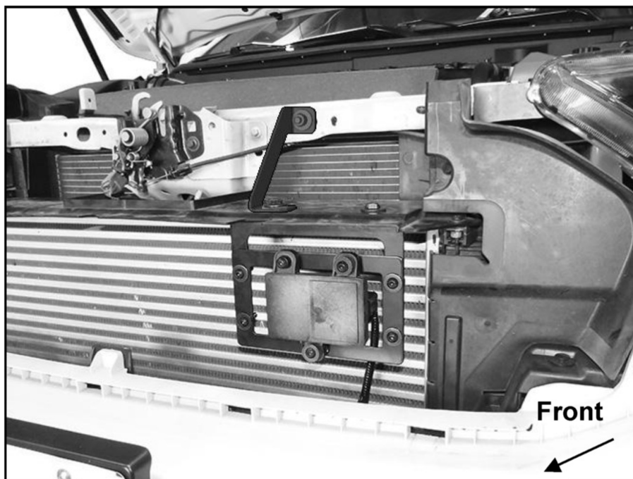
(Fig 32) Ranger Models. Plug harness into sensor. Check sensor alignment before tightening hardware
