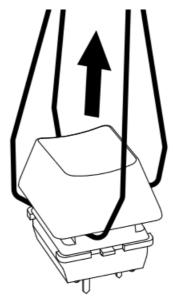
**Step 02**Remove the switch with switch puller side of the tool.
