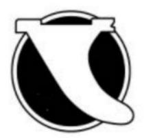
Insert fin into a notched section of fin box first then rock fin towards the rear of the board until fin is seated completely in the fix box. Lock fin into place by flipping the lever lock down into the locking position. Repeat steps for 2 outer fins.
