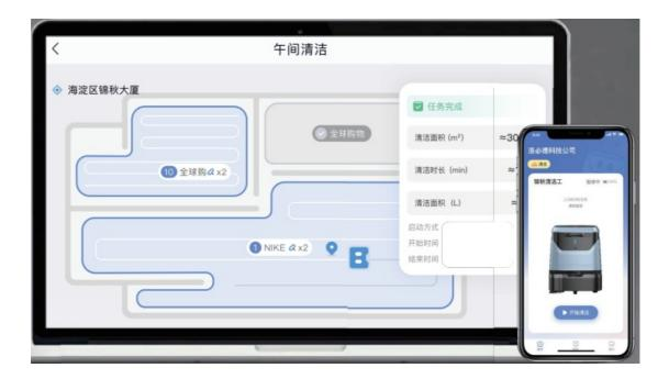
You can assign cleaning tasks for designated spots at fixed times to the robot through its screen, the cloud platform, or the app.
